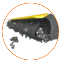
Milling cutter with cross knives system
